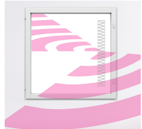
Figure 3: The surface of the glass features a discreet antenna pattern. The patent-protected solution facilitates the transfer of signals into the dwelling.
